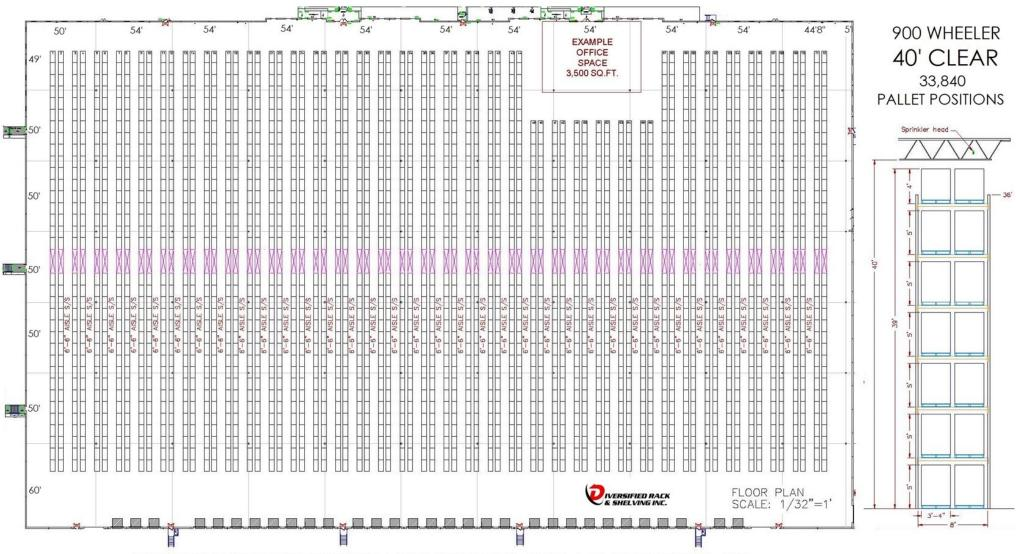
6'-6" VNA AISLES | WIRE GUIDANCE FORKLIFT | 2,376 - 8' BAYS (X14PP = 33,264) | 72 - 17' TUNNELS (X8PP = 576)
